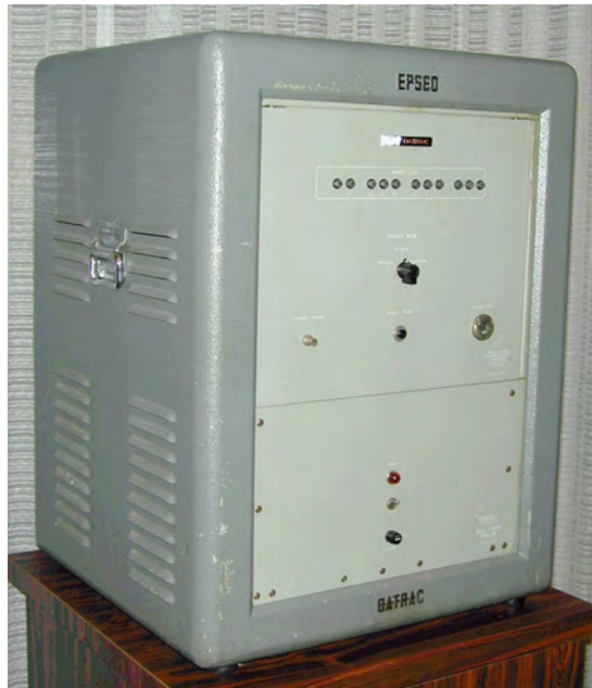
Figure 3.62: 1954 "DATRAC" 11-Bit, 50-kSPS SAR ADC Designed by Bernard M. Gordon at EPSCO
